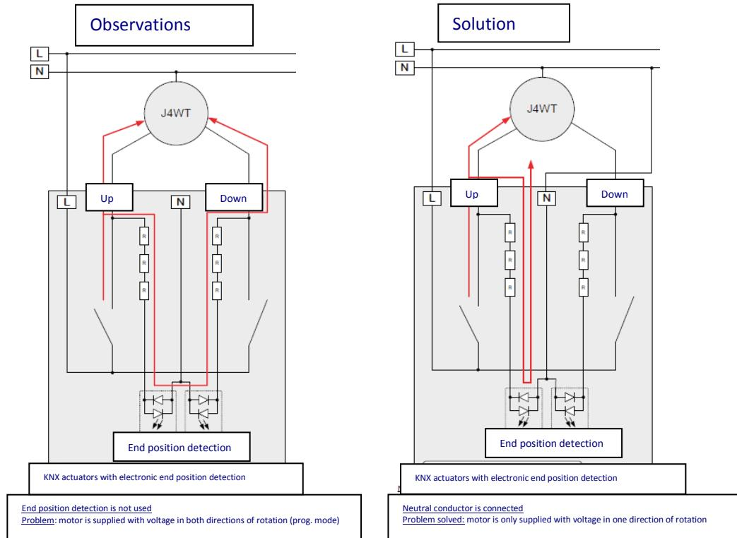
The neutral conductor connection on the actuator serves as a necessary measuring point. In this case, every N-terminal (measuring point on the actuator) and every drive neutral conductor must be routed on neutral conductor potentials (N rails).
