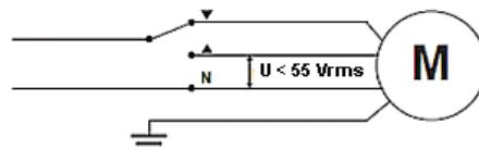
9. Somfy WT drives may not be operated using a solid state relay.
