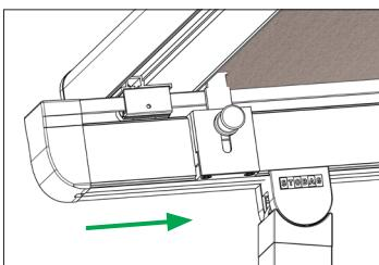
▴ Retract the awning to the front rail locking mechanism by pressing the UP button until the motor stops.
