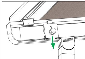
Release all front-rail locking mechanisms (on both sides and on all guide rails).
