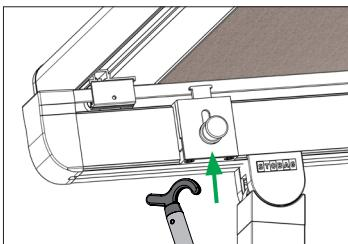
Fasten all front-rail locking mechanisms (on both sides and on all guide rails).
