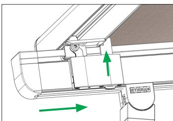
2. The awning retracts and the locking mechanism is automatically fastened, tensioning the awning fabric.
