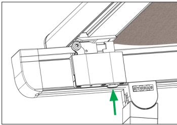
With the sliding element against the ramp, reattach the draw hook.
